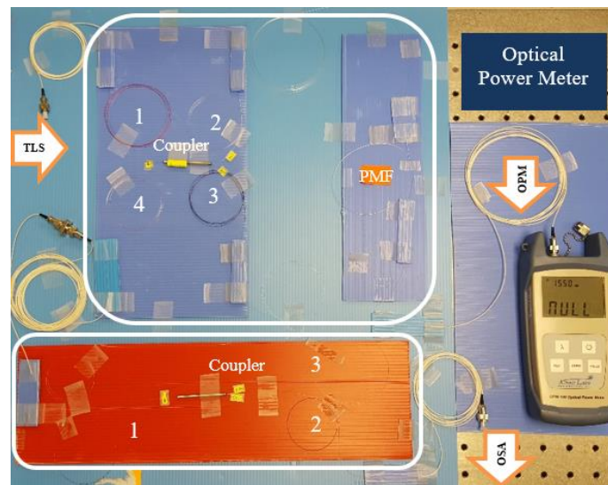
Figure 2: Actual experimental setup of laser scanning technique using TLS on the optical breadboard
